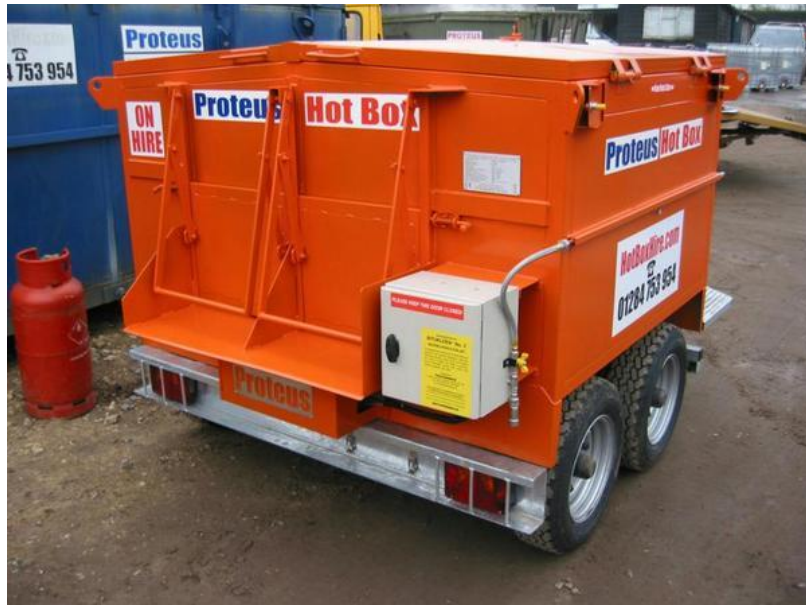
Figure 8. Asphalt hot box (photo courtesy of Proteus).
