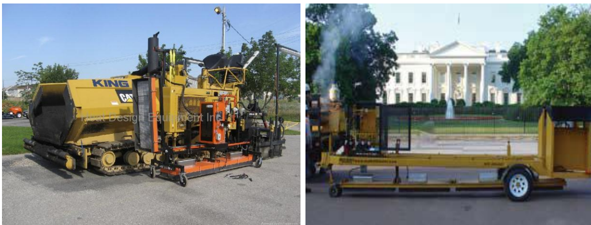
Figure 23. Joint heater (photo courtesy of Heat Design Equipment Inc.)
