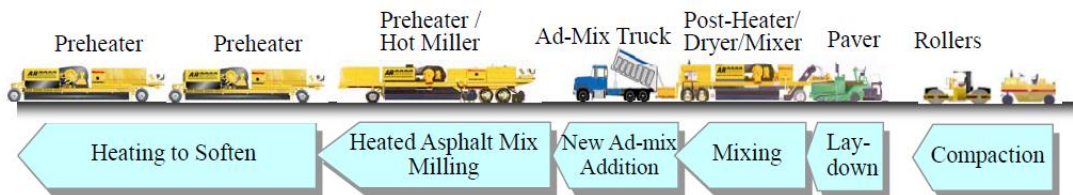
Figure 15. Hot in-place recycling (Hosokawa et al, 2005)
