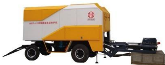
Figure 25 Trailer mounted microwave unit (photo courtesy of New Timehope)
