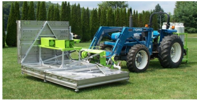
Figure 14. Infra-red heater fixed to a tractor
