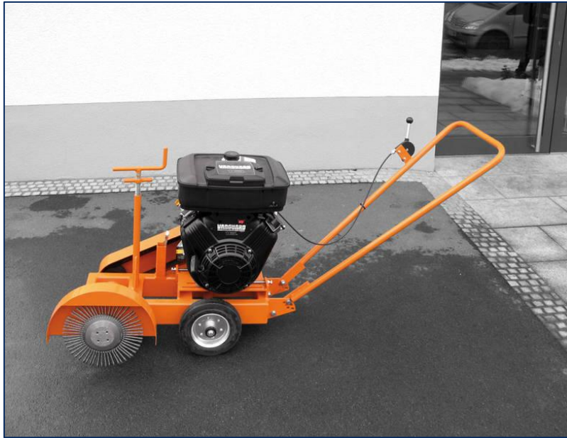
Figure 6. Joint brushing machine (photo courtesy of Schafer Technic)
