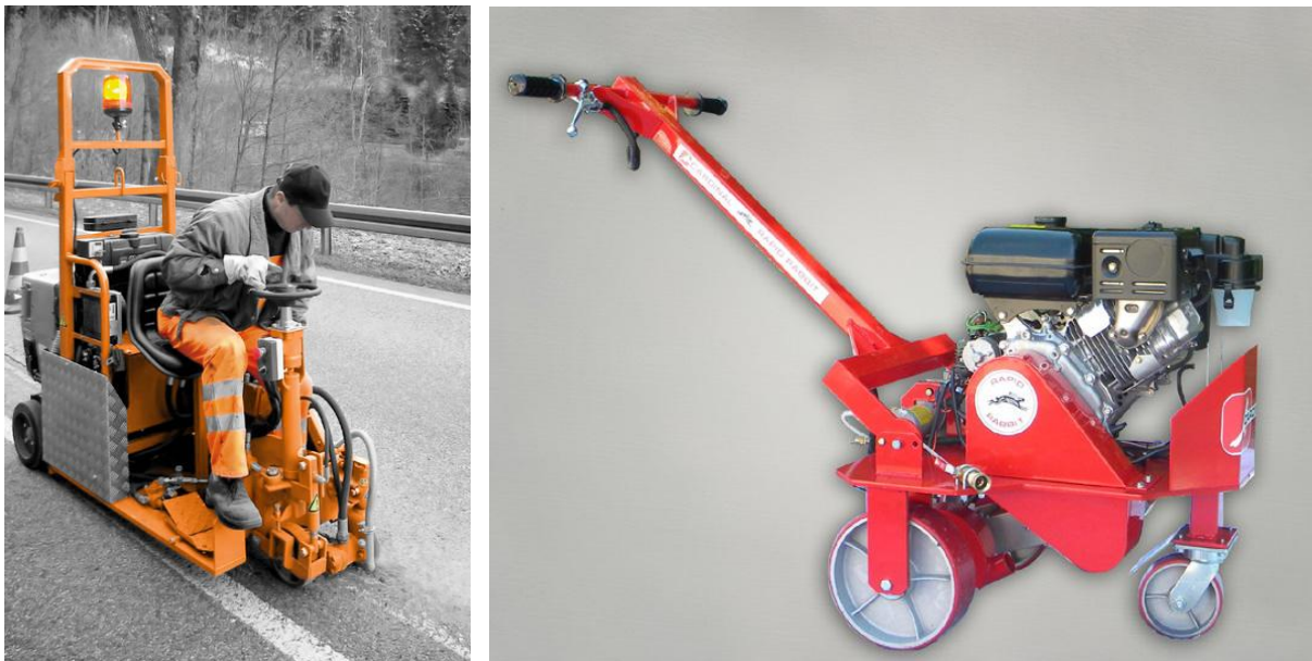
Figure 5. Crack chaser (photo courtesy of Cardinal) and Joint milling machine (photo courtesy of Schafer Technic)
